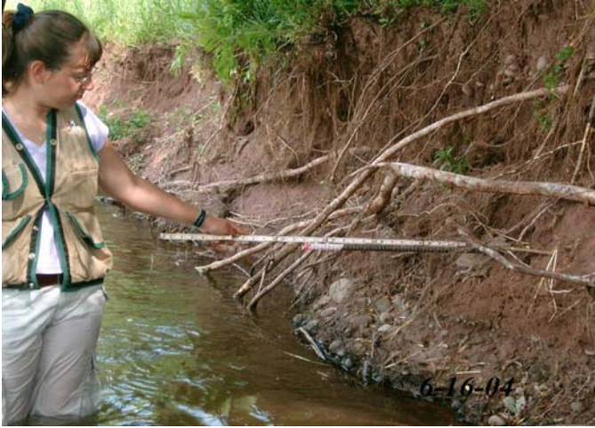
Figure 7.3.14 Monitor bank pin located in the eroding bank that is shown in the Figure 7.3.15 .
